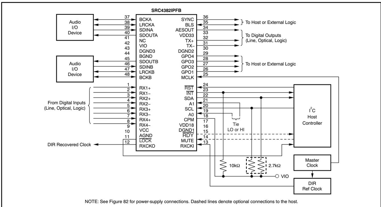
**Figure 81. Typical Application Diagram Using I<sup>2</sup>C Host Interface**
