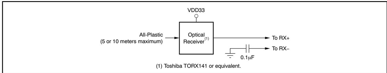
Figure 85. Interfacing to a +3.3V Optical Receiver Module
