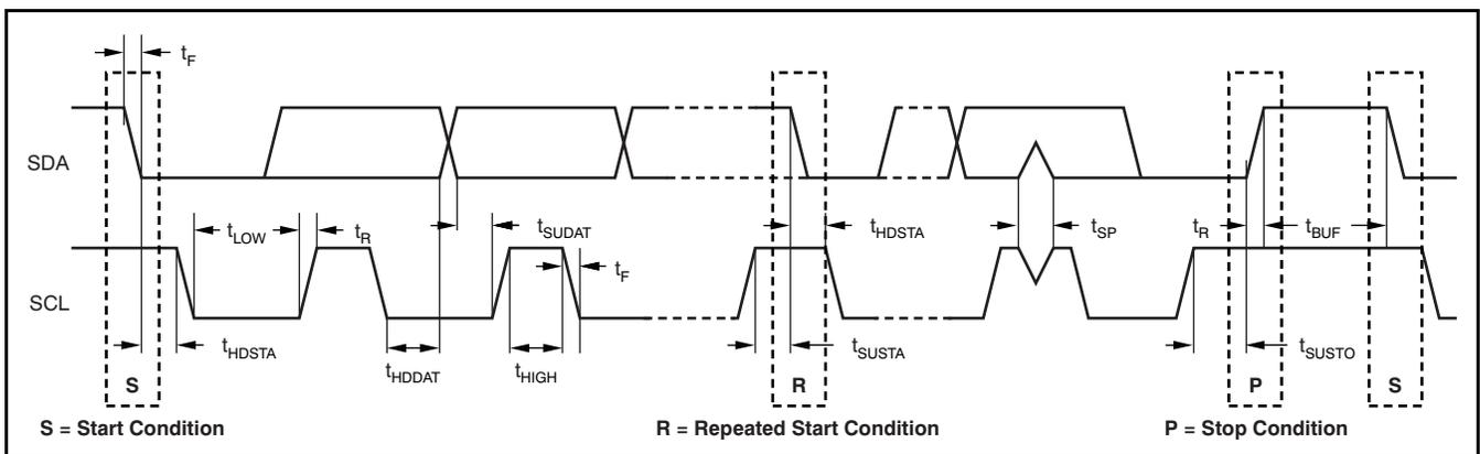
**Figure 3. I<sup>2</sup>C Standard and Fast Mode Timing**
