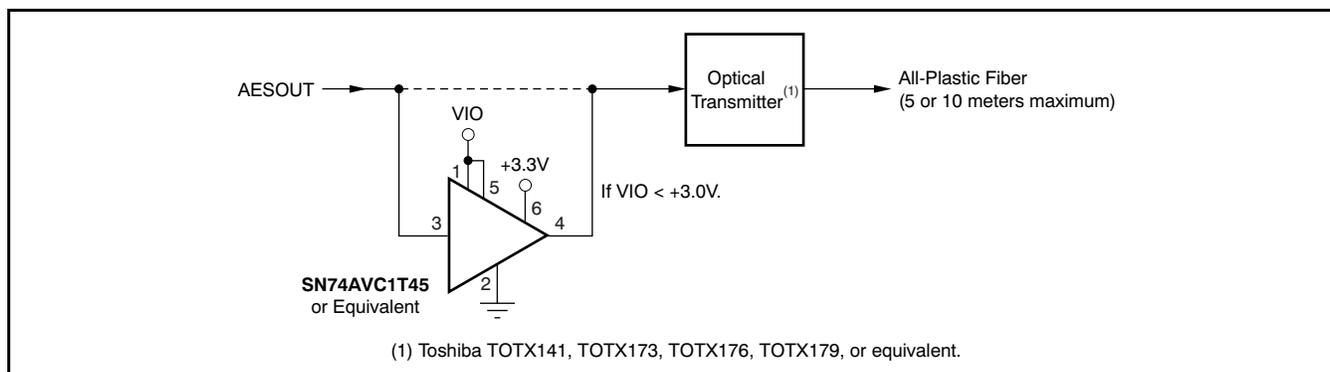
**Figure 90. Interfacing to an Optical Transmitter Module**
