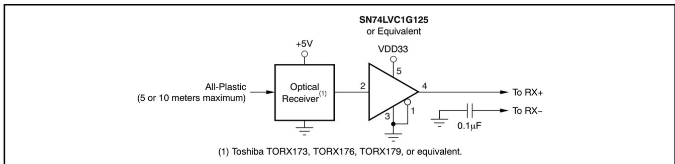
Figure 86. Interfacing to a +5V Optical Receiver Module
