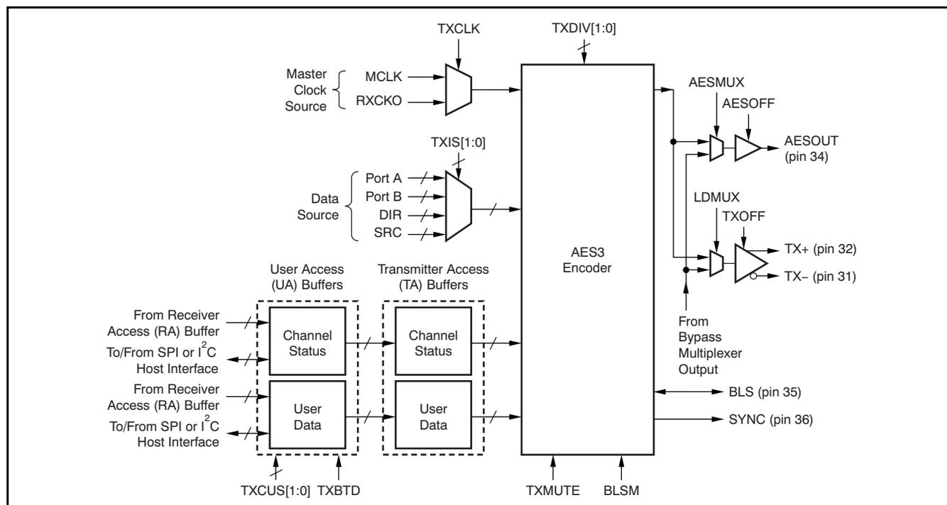
**Figure 65. Digital Interface Transmitter (DIT) Functional Block Diagram**
