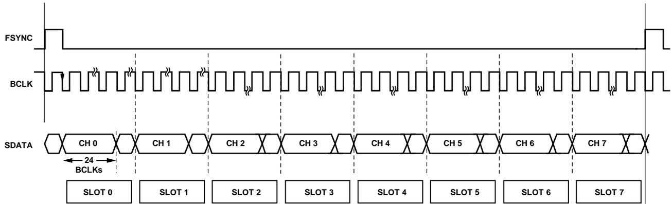
Figure 21. TDM-8 Hardware Mode, SCL = 1, SDA = 0, I<sup>2</sup>C Mode, One BCLK Delay, Normal Clock Polarity, Default Channel Assignments
