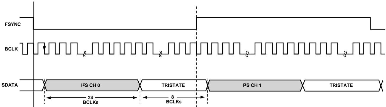
Figure 18. SPT\_SIA\_MODE = Stereo Mode (I²S), I²C Operation Only
