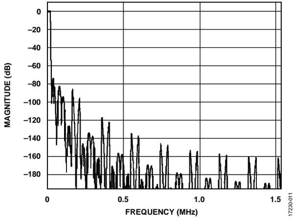
Figure 10. Magnitude vs. Frequency, 48 kHz Output, 64x Decimation
