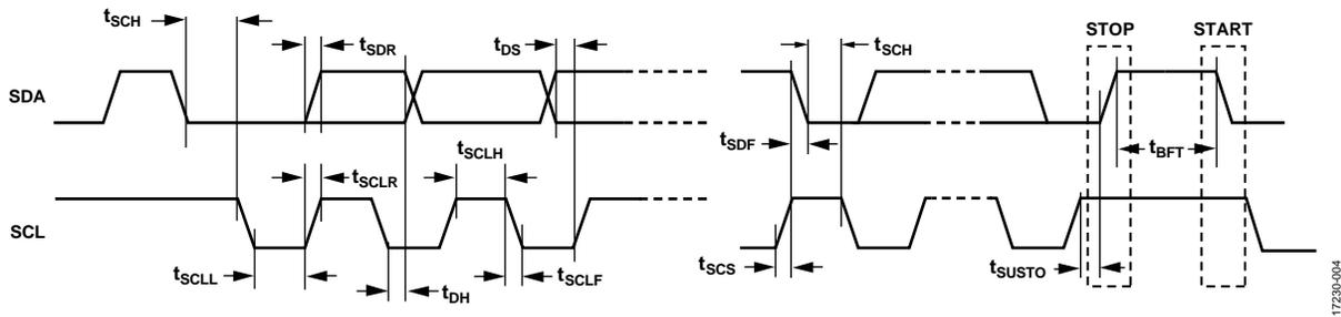
Figure 3. I<sup>2</sup>C Slave Port Timing Specifications
