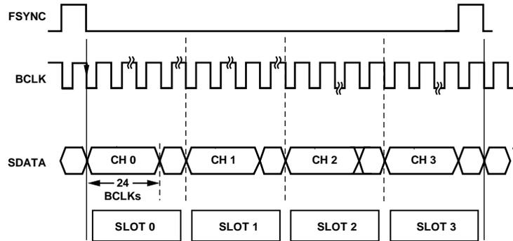
Figure 23. TDM-4, Hardware Mode, SCL = 1, SDA = 1, I<sup>2</sup>C Mode, One BCLK Delay, Normal Clock Polarity, Default Channel Assignments
