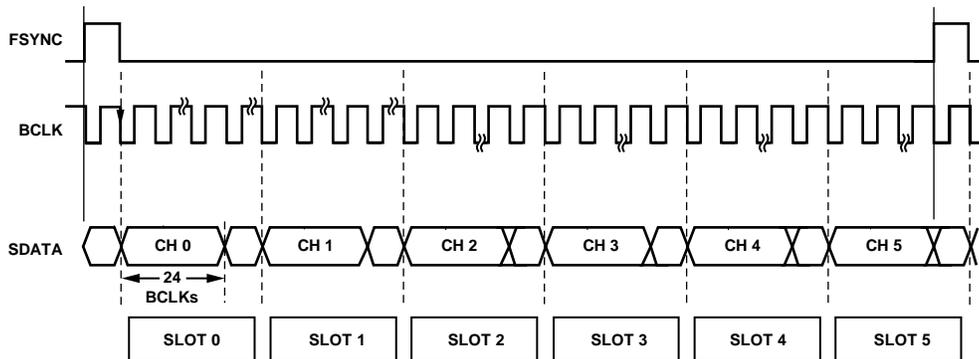
Figure 22. TDM-6, Hardware Mode, SCL = 0, SDA = x, I<sup>2</sup>C Mode, One BCLK Delay, Normal Clock Polarity, Default Channel Assignments
