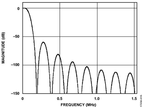
Figure 14. Magnitude vs. Frequency, 48 kHz Output, 16x Decimation
