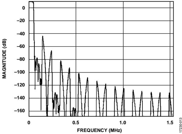
Figure 12. Magnitude vs. Frequency, 48 kHz Output, 32x Decimation
