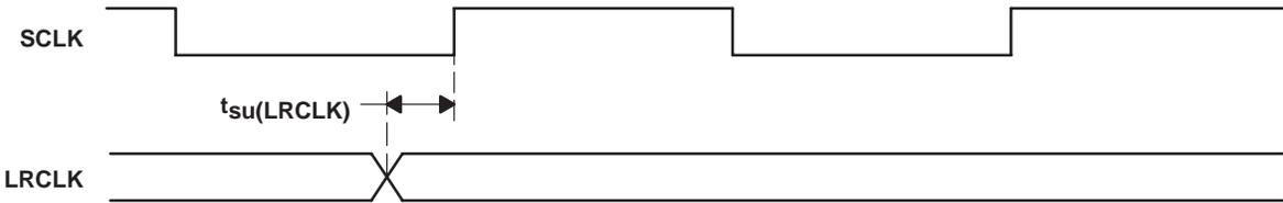
NOTE: Serial data is sampled with the rising edge of SCLK (setup time = 20 ns and hold time = 10 ns)
