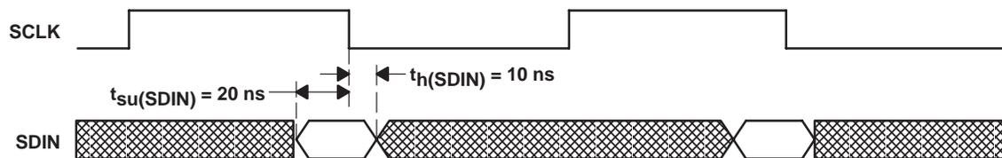
NOTE: Serial data is sampled with the falling edge of SCLK (setup time = 20 ns and hold time = 10 ns)
