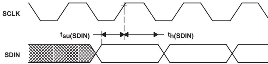
Figure 11. Right-Justified, IIS, Left-Justified Serial Protocol Timing
