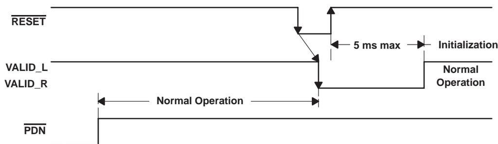
Figure 3. Reset Timing
