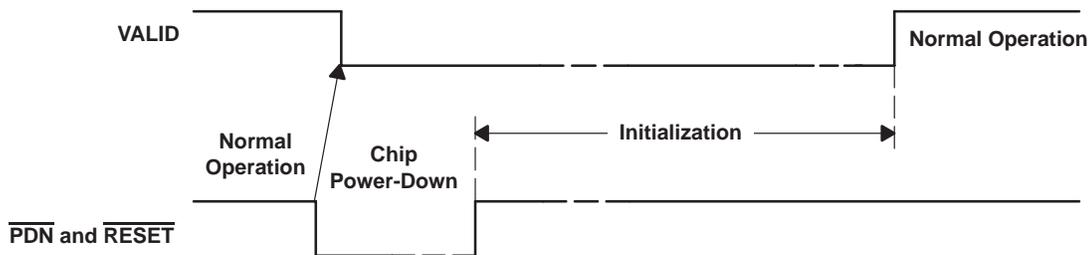
Figure 4. Power-Down Timing
