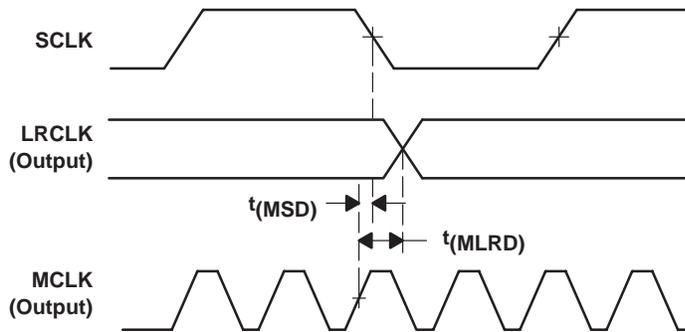
Figure 13. Serial Audio Ports Master Mode Timing
