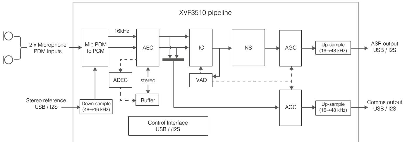
Figure 1: XVF3510 block diagram
