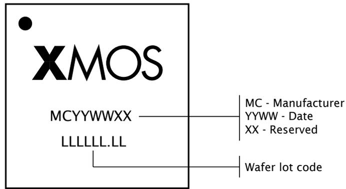
Figure 13: Part marking scheme
