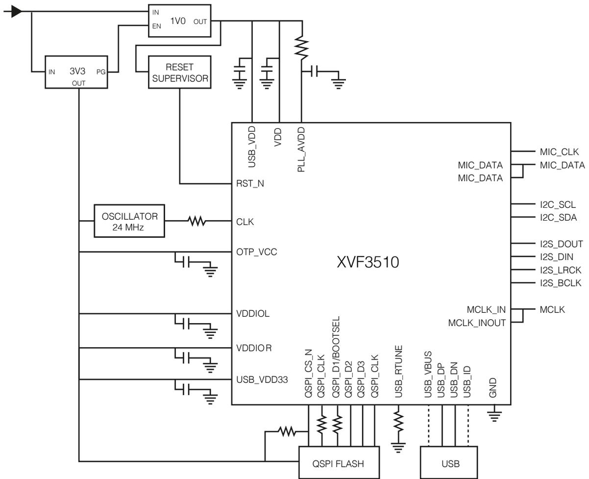
Figure 2: XVF3510 example application diagram
