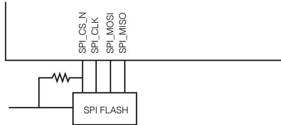
Figure 4: XVF3510 SPI pins
