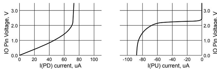
Figure 14: Typical internal pull-down and pull-up currents
