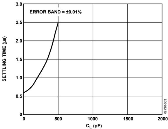
Figure 63. OPA627 Settling Time vs. Load Capacitance
