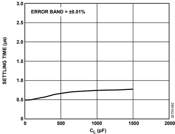
Figure 62. AD8610/AD8620 Settling Time vs. Load Capacitance
