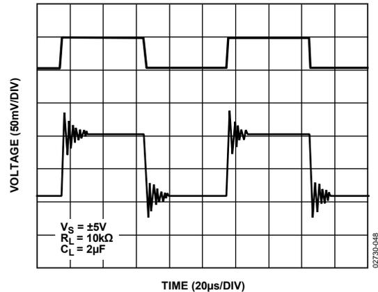
Figure 48. AD8610/AD8620 Capacitive Load Drive,  $A_V = +2$
