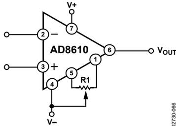
Figure 66. Offset Voltage Nulling Circuit
