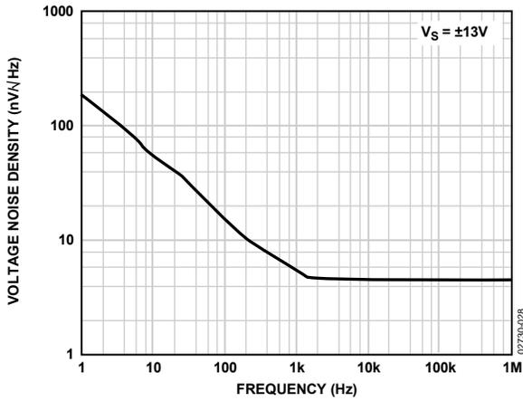
Figure 28. Input Voltage Noise Density vs. Frequency
