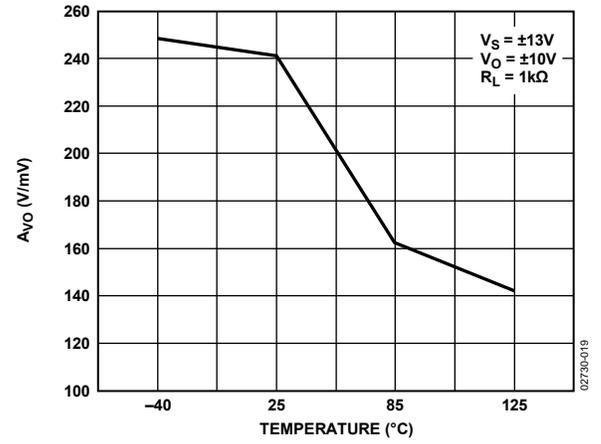
Figure 19. A<sub>vo</sub> vs. Temperature
