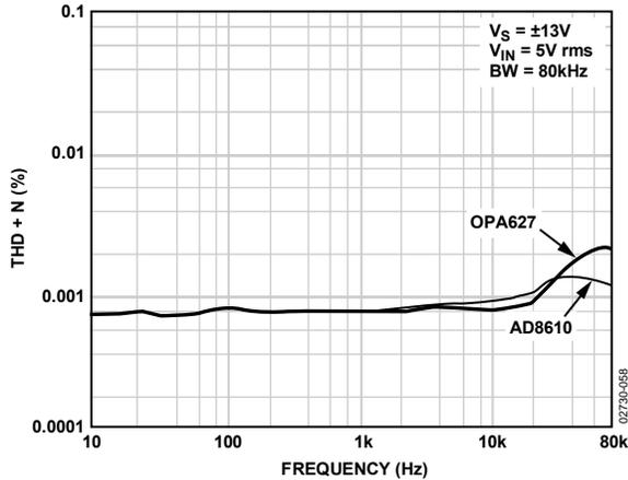
Figure 58. AD8610 vs. OPA627 THD + Noise @  $V_{CM} = 0 V$
