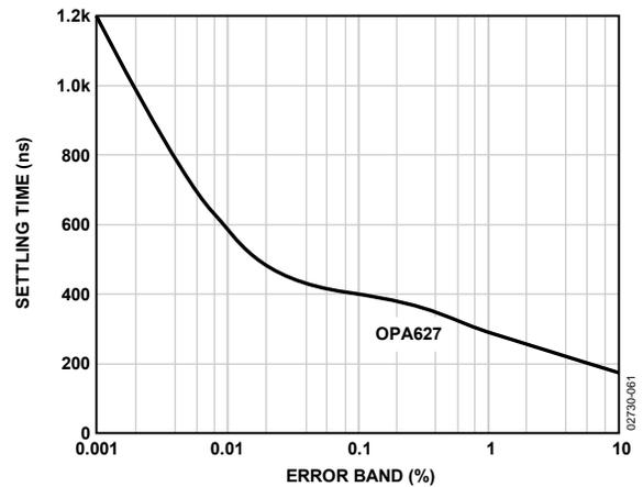
Figure 61. OPA627 Settling Time vs. Error Band
