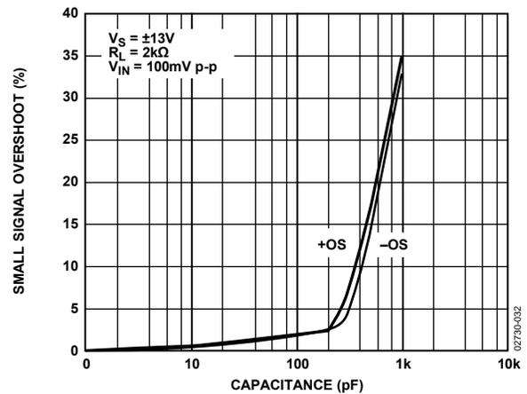
Figure 32. Small Signal Overshoot vs. Load Capacitance
