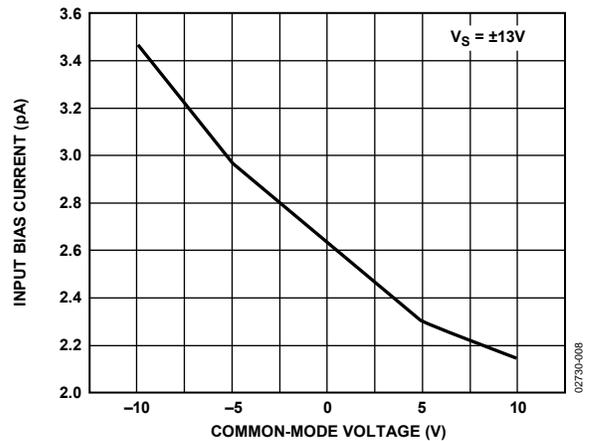
Figure 8. Input Bias Current vs. Common-Mode Voltage
