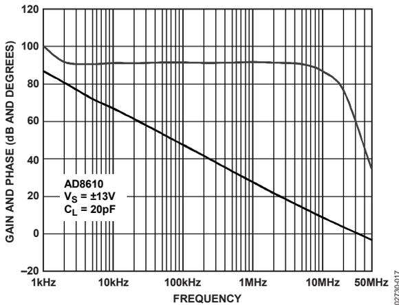
Figure 17. Open-Loop Gain and Phase vs. Frequency
