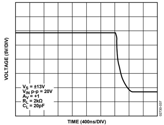
Figure 37. -Slew Rate at  $G = +1$
