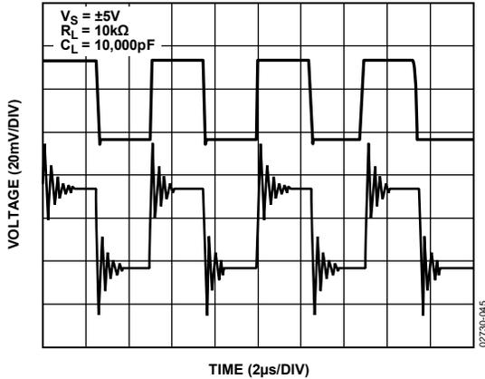
Figure 45. AD8610/AD8620 Driving  $C_L = 10,000$  pF
