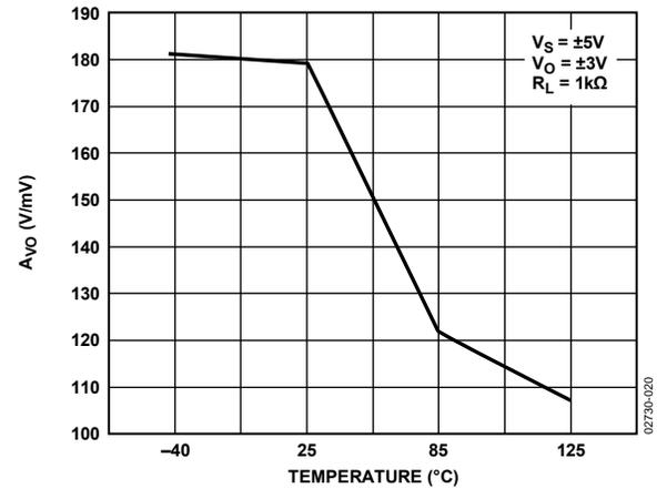
Figure 20. A<sub>vo</sub> vs. Temperature
