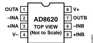
Figure 2. 8-Lead SOIC\_N
