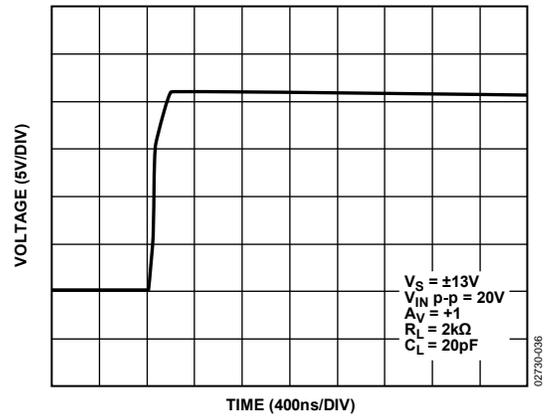
Figure 36. +Slew Rate at  $G = +1$
