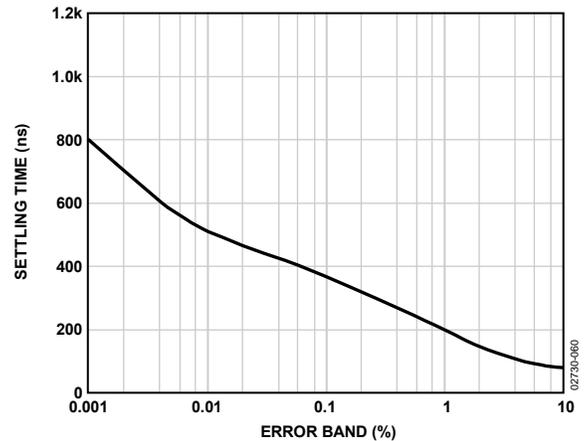
Figure 60. AD8610/AD8620 Settling Time vs. Error Band
