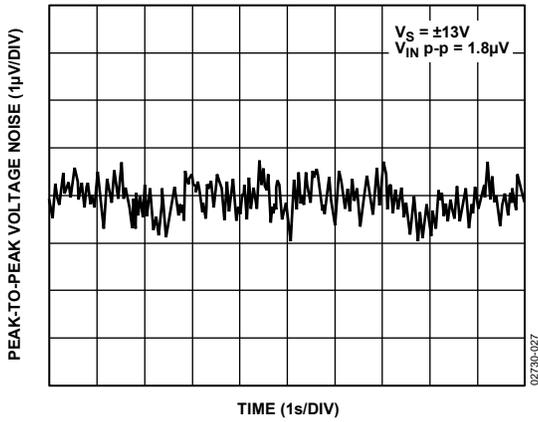
Figure 27. 0.1 Hz to 10 Hz Input Voltage Noise
