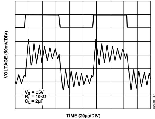
Figure 47. OPA627 Capacitive Load Drive,  $A_V = +2$
