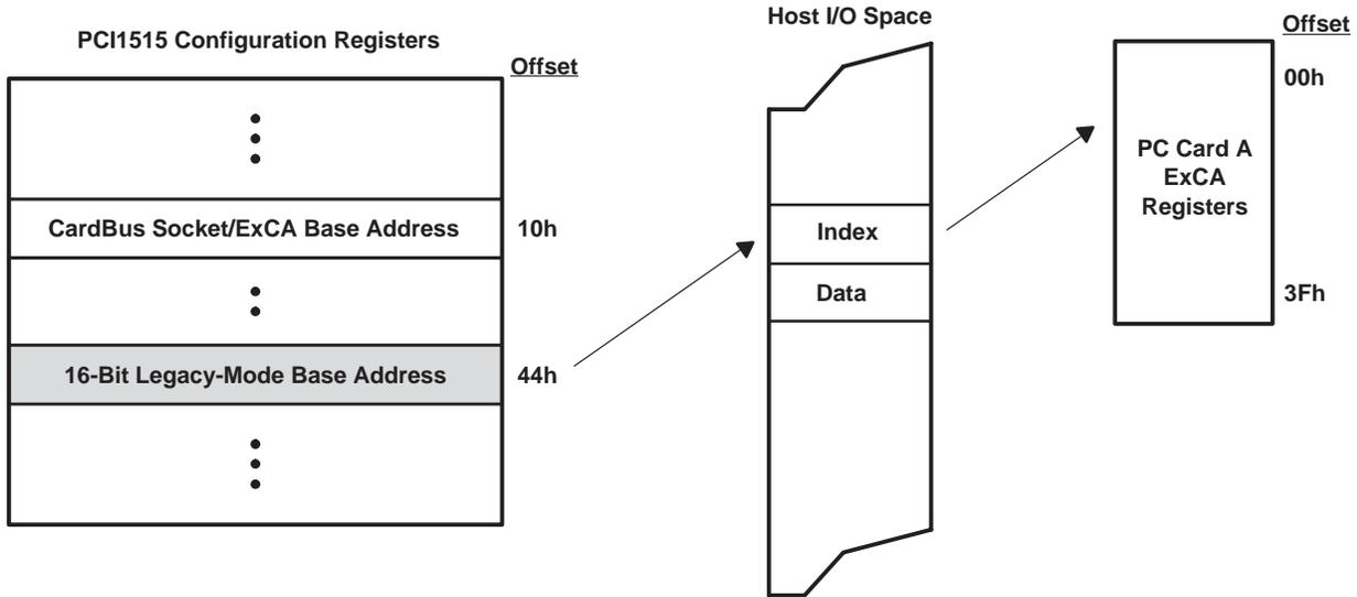
Offset of desired register is placed in the index register and the data from that location is returned in the data register.
