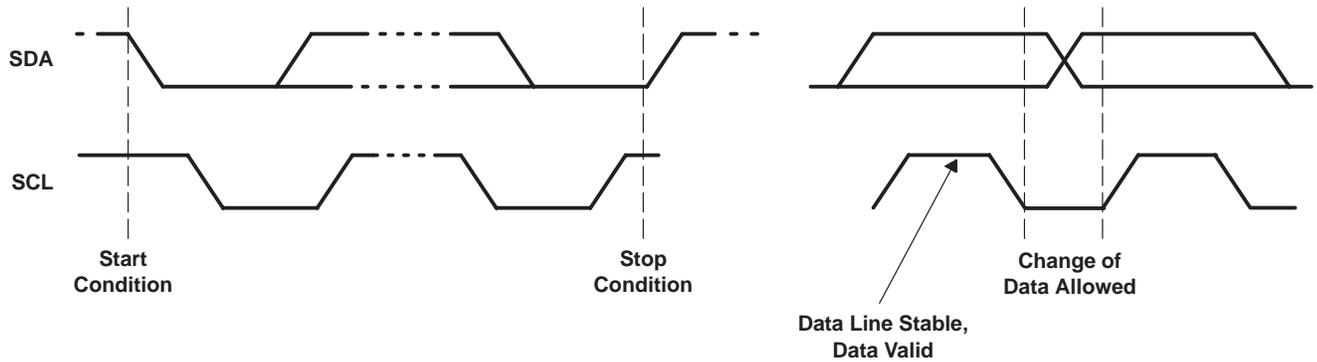
**Figure 3–6. Serial-Bus Start/Stop Conditions and Bit Transfers**
